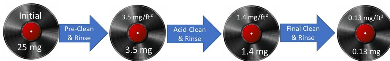
**Figure 41 – Record NVR Following Precision Aqueous Cleaning Process**
