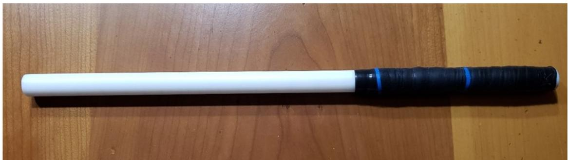
**Figure 32 – Teflon Rod w/Silicone Tape**
