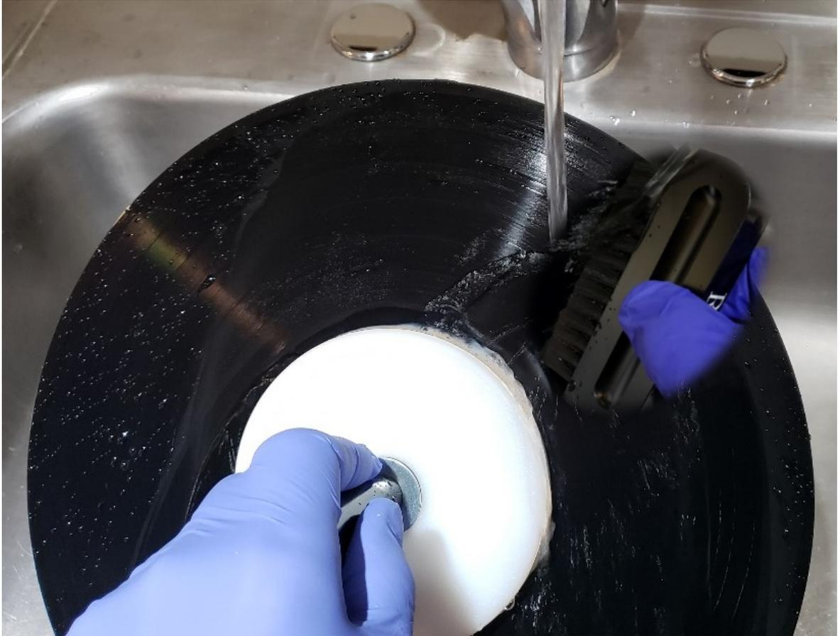
**Figure 20 – Step 7: Acid Rinse with Tap Water & Brush**
