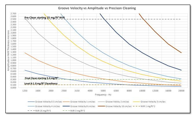
Figure 46 - Groove Velocity vs Amplitude vs Contamination Levels
