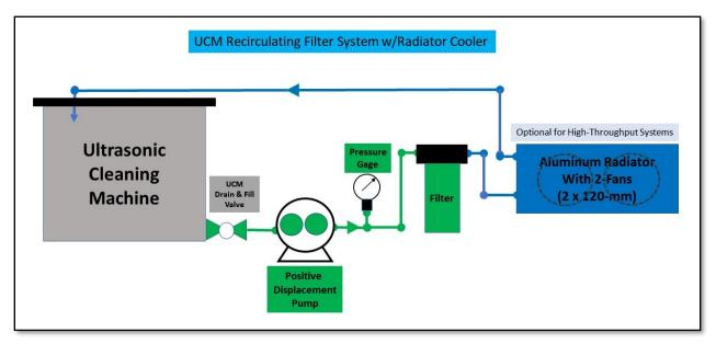
Figure 58 - UCM Recirculating Filter System w/Radiator Cooler
