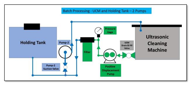
Figure 59 - Batch Processing UCM and Holding Tank - 2 Pumps
