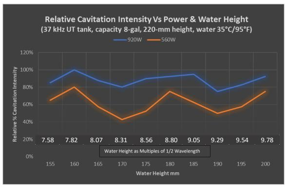
Figure 54 - Relative Cavitation Intensity vs Power & Water Height
