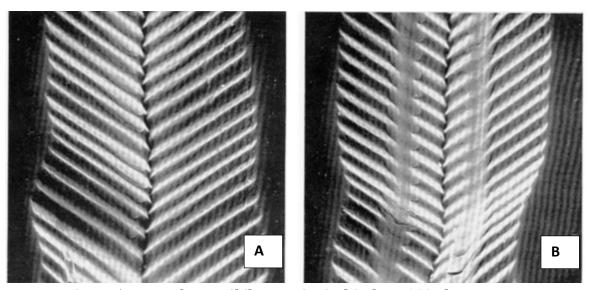
Figure 5 – Record Wear Shibata vs Conical Stylus – 100 Plays (Image Development of Compound for Quadradiscs, G.A. Bogantz & S.K. Khanna, RCA 1976 "scan courtesy of www.worldhistory.com")
