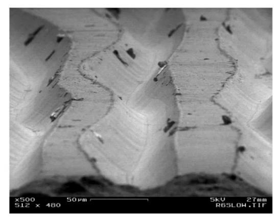
Figure 48 – Record Groove Magnified 500X (Image courtesy of University of Rochester: URnano)
