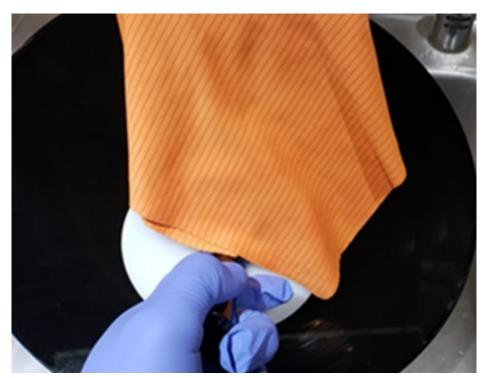
Figure 25 – Step 12: Drying with Kinetronics™ Anti-static Cloth
