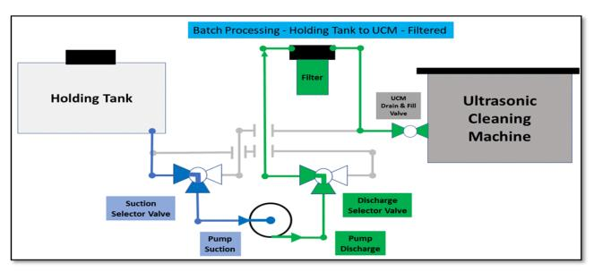
Figure 61 - Batch Processing - Holding Tank to UCM - Filtered
