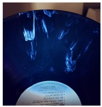
Figure 9 - One Record Inspected UV Light - Heavily Soiled with Staining
