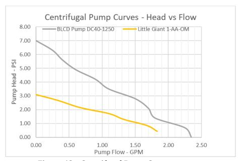
Figure 62 - Centrifugal Pump Curves
