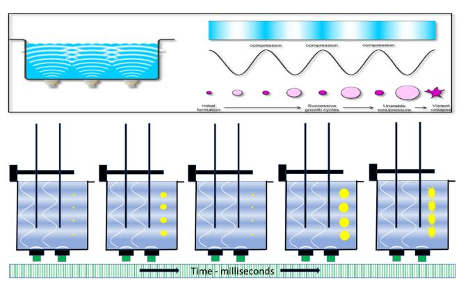
Figure 52 - Fundamentals of Ultrasonic Cavitation
