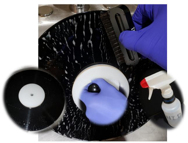
Figure 21 - Step 8: Final Clean with NID Solution & Brush
