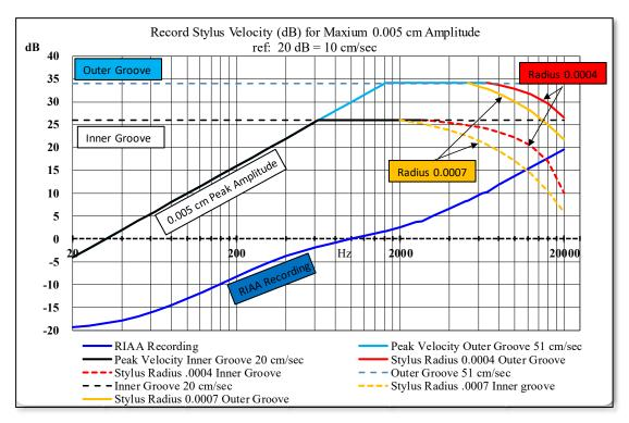
Figure 44 - Record Groove Velocity
