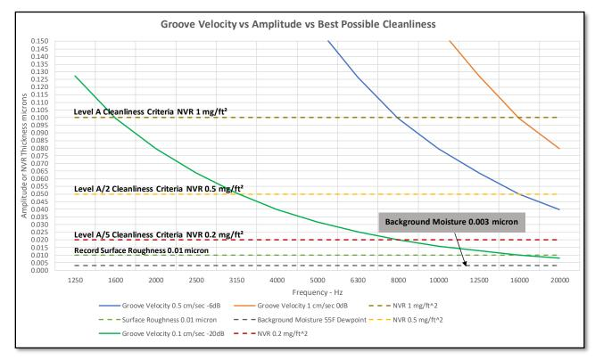
Figure 47 - Groove Velocity vs Amplitude vs Best Possible Cleanliness
