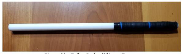
Figure 32 - Teflon Rod w/Silicone Tape
