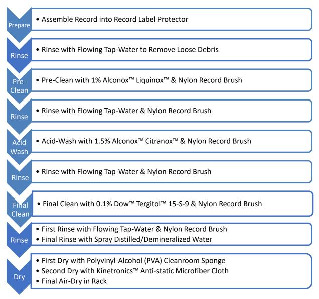
Figure 6 - Precision Aqueous Vinyl Record Cleaning Process Summary
