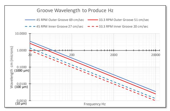
Figure 42 - Record Groove Wavelength to Produce Hz
