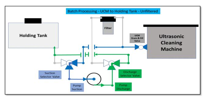
Figure 60 - Batch Processing - UCM to Holding Tank - Unfiltered
