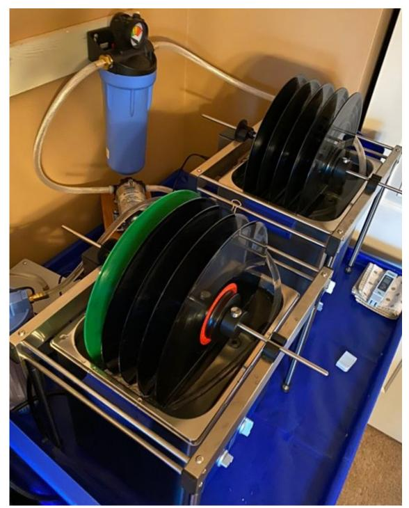
Figure 56 - Elmasonic™ UCM Filtered Clean/Rinse System & Kuzma™ Spinner w/Records
