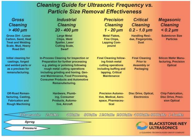
Figure 53 - UT Tank Frequency Cleaning Guide
