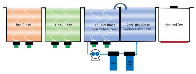
Figure 49 - Industrial Precision Ultrasonic Cleaning Console
