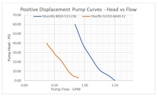
Figure 63 - Positive Displacement Pump Curves
