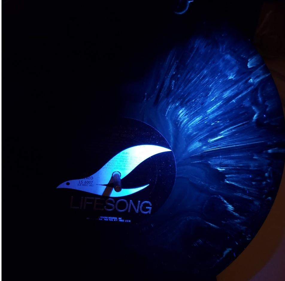
**Figure 10 – Record Inspected UV Light – with Major Staining**
