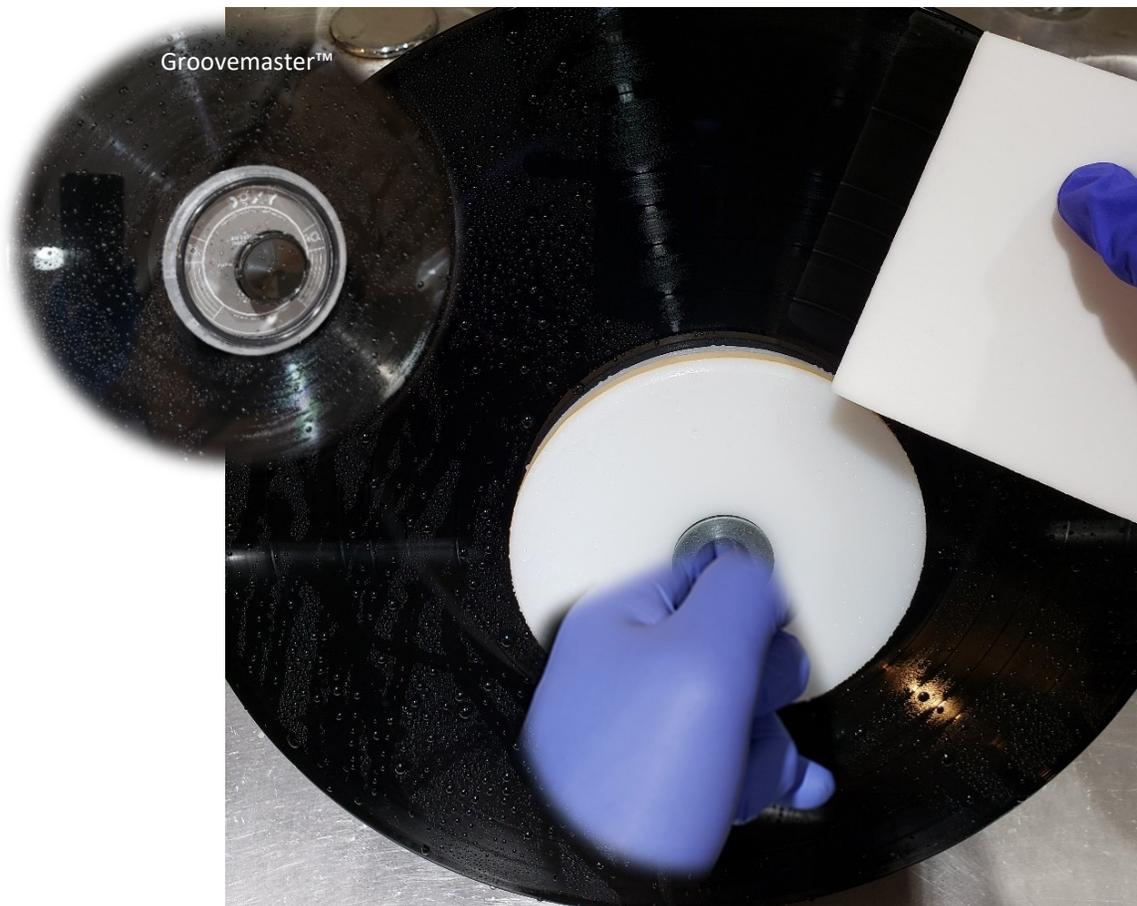
**Figure 24 – Step 11: Drying with Super Cool™ PVA Cleanroom Sponge**
